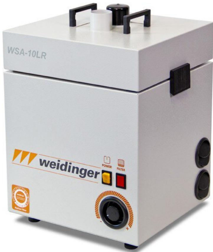
The WSA-10LR extraction unit for solder fumes has 2 extraction ports with an outer diameter of 50 mm (top), 4 adjustable blow-out gills (both sides, bottom), an optical filter indicator and a volume flow controller.
