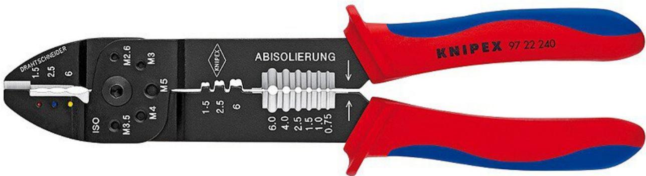
For cable cutting, wire stripping and crimping of insulated and uninsulated cable lugs and connectors and open connectors. With threaded holes for cutting Cu or Ms threaded pins with M 2.6; M 3; M 3.5; M 4 and M 5. Screwed joint for high stability and smooth running. - Application: insulated cable lugs + cable connectors/uninsulated, open connectors (6.3 mm plug width) - Capacity square millimetres: 0.5 - 6.0mm<sup>2</sup> - Number of nests: 3 - AWG: 20 - 10
