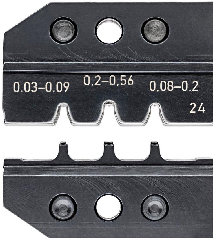
Application: D-Sub, HD 20, HDE connectors 0.03 - 0.56 mm<sup>2</sup>. - Nominal size: 0.03 - 0.56 mm<sup>2</sup> - Application: D-sub; HD 20-; HDE-connectors - Capacity square millimeter: 0.03 - 0.56mm<sup>2</sup> - Number of nests: 3 - AWG: 32 - 20.
