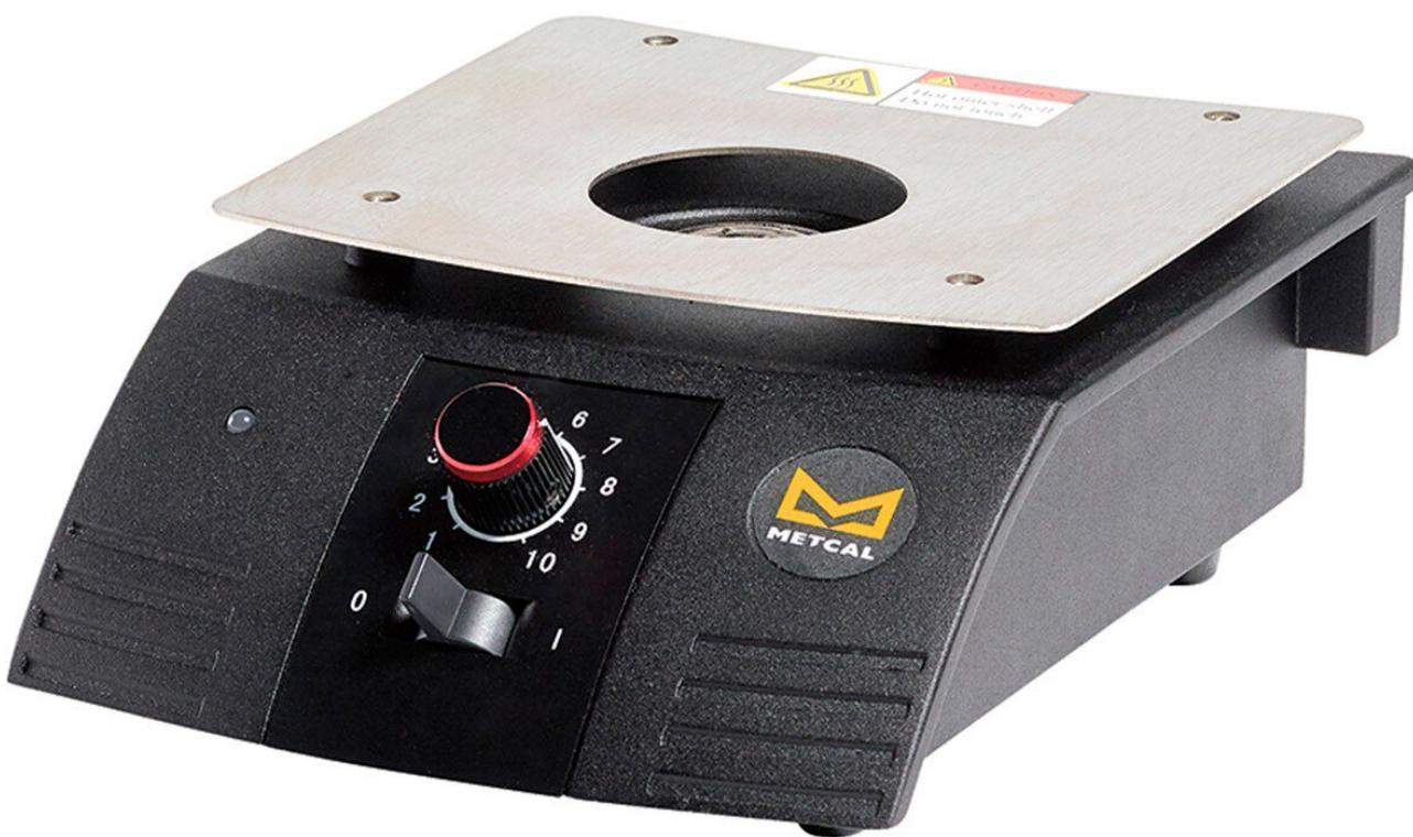
The PCT-100 Focus Pre-heater targets heat for improved speed and efficiency for high thermal demand applications, including lead-free. Used for SMT and through-hole hand processes, the PCT-100 uses convection air heating to heat a PCB first, for better soldering, improved process control and increased productivity. The PCT-100 Focus Pre-heater adds heat volume, without turning up the temperature, to perform assembly tasks at the appropriate peak temperature without distorting the board.
