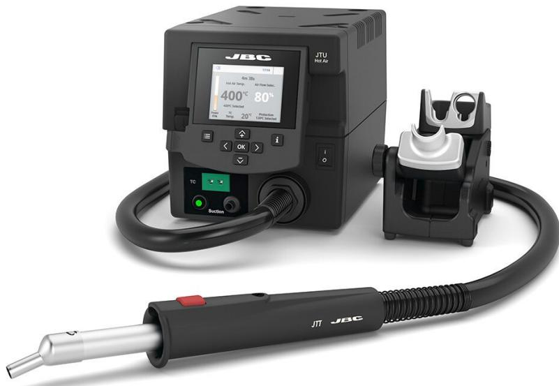
The JBC JTSE-2QB hot air soldering station is a powerful and precise solution for the repair and rework of SMD components, including complex QFPs and PLCCs. With a rated power of 700 W and a temperature range of 150°C to 450°C, it enables fast and safe desoldering. The airflow control from 5 to 50 SLPM ensures a smooth and controlled airflow, ideal for demanding applications.
