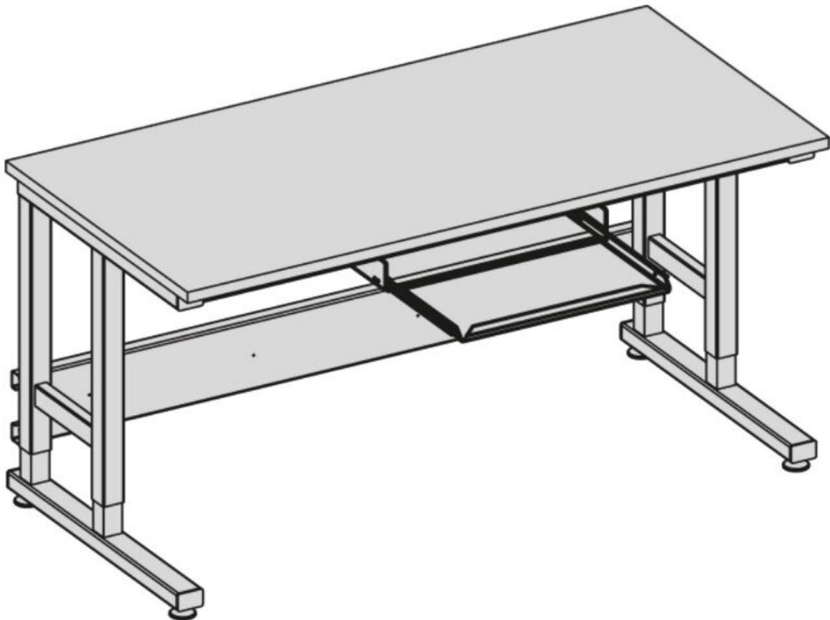
The keyboard drawer can be mounted on both sides and adjusted in height to ensure an ergonomic working position.
