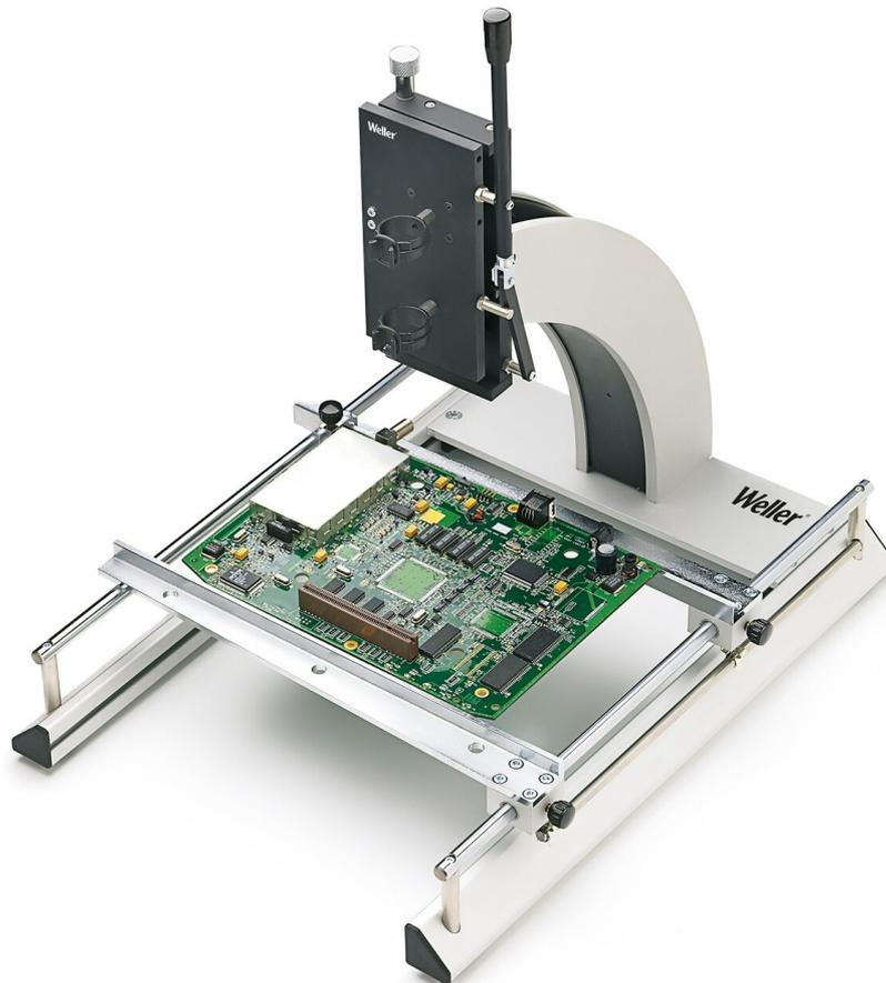
The WBHS PCB holder from Weller is specially designed for use with the WHA 3000P, WHA 3000V and WTHA 1 models. It offers a heated area of 80 x 50 mm (3.15 x 1.97 inches) and is equipped with a precise platinum sensor. The internal parameter memory ensures reliable and consistent performance without tolerance deviations. This product is ideal for applications that require stable and precise handling of PCBs.
