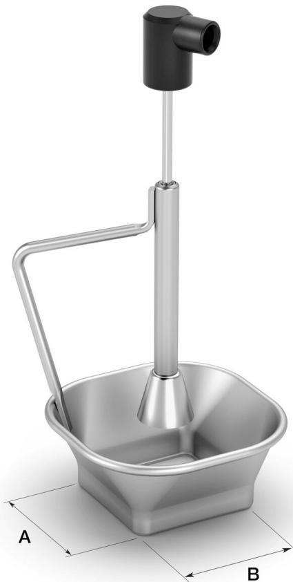
The vacuum puller with protective cup, PLCC 80, 24 x 24 mm, is the ideal addition to hot air repair stations. This protective device enables precise work by concentrating the heat on the desired area and protecting adjacent components at the same time. The integrated vacuum puller ensures efficient handling and facilitates the removal of components.
