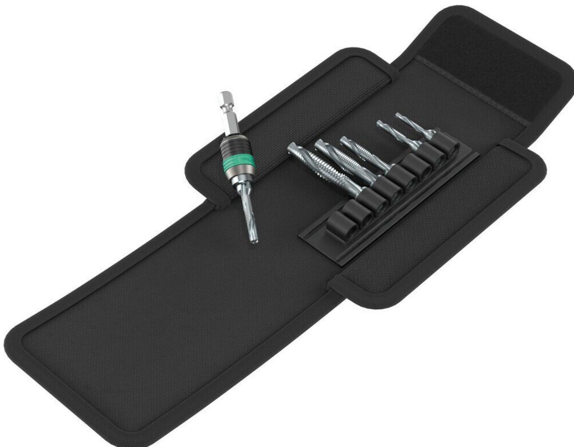
7-piece combination tap bit set from Wera in robust folding case 9570. 1/4" drive suitable for holders to DIN ISO 1173-D 6.3. With Rapidaptor quick-change holder for mounting in the screwdriver or for use in the chuck of the electronic drill. Very good power transmission due to hexagonal shank. HSS = high speed steel. Finely tuned material elasticity for long tool life. Very good centering properties. Problem-free cutting. Perfect chip removal. Low risk of jamming. Precise return guidance.
