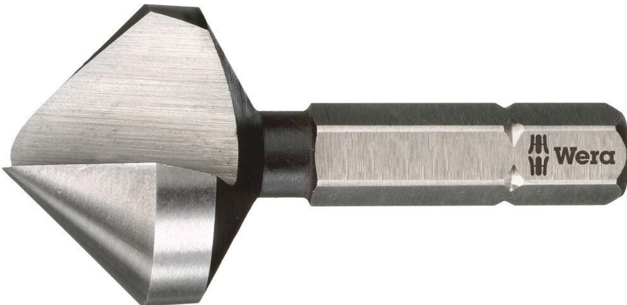
High-quality 1 flute countersink bit from Wera. For countersinking and deburring. The hexagonal shank ensures very good power transmission. Guaranteed chatter-free and scoring-free work. Perfect chip removal and long tool life. 1/4" hexagon, suitable for DIN ISO 1173-D 6.3 holders.
