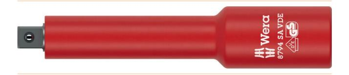
1/4" VDE extension with increased safety due to yellow insulation core, which becomes visible if the outer red VDE insulation layer is damaged. Unit-tested tool in accordance with IEC 60900 at 10,000 V for safe working at the approved voltage of 1,000 V.
