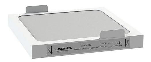
The FAE1-110 pre-filter protects the HEPA filter H13 and extends its service life. The combination of the three-layer filter system achieves a certified filter efficiency of up to 99.95 % for soldering fumes in accordance with the EN 1822 standard. The device also has an LED warning indicator that shows when the pre-filter or compact filter needs to be replaced. A corresponding message is also shown on the device display.
