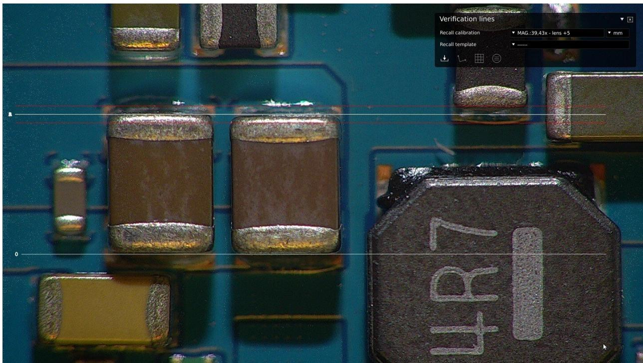
For products with strict size and distance requirements, the Verification Lines app allows you to superimpose lines with user-defined tolerances over the microscope image. The overlaid, accurately calibrated verification lines make it easy to perform outgoing inspections or other forms of visual inspection.
