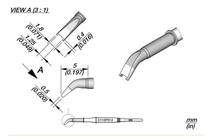
C115 cartridges are appropriate for desoldering chip components.
