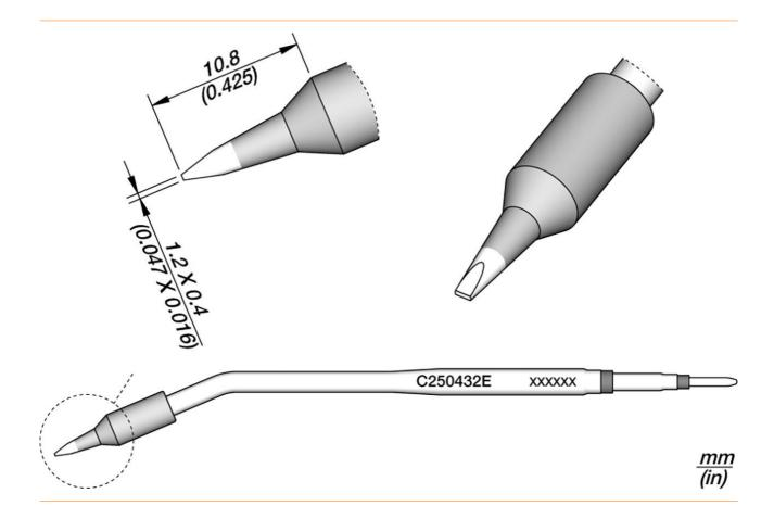
This cartridge was developed with a thicker iron layer, which makes this tip ideal for hard and repetitive work in mass production. A thicker iron layer reduces thermal efficiency. The C250 cartridges have been specially developed for use with the ALE250 automatic feed soldering iron and the AP250 manual feed soldering iron.
