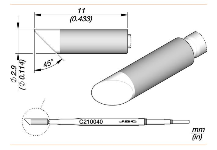
The C210 cartridges are suitable for precision soldering work with medium power requirements.
