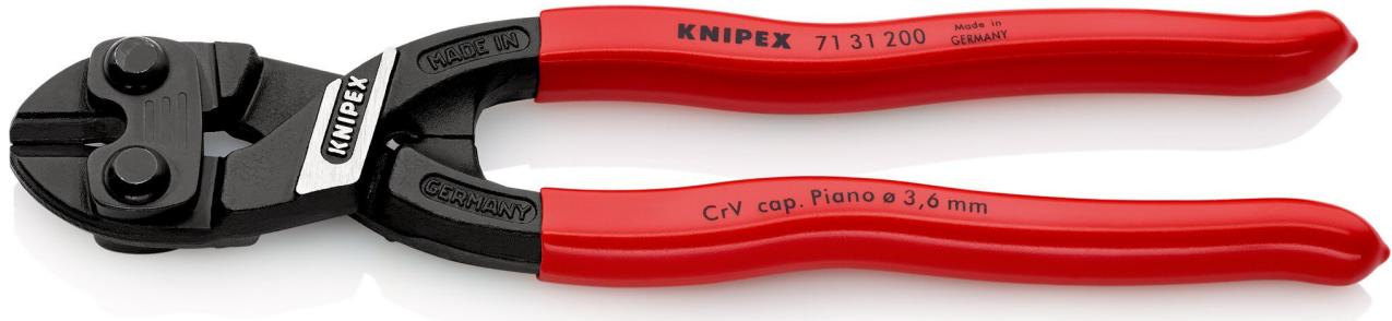
With precision cutting edges for soft, hard wire as well as piano wire. Cuts components such as bolts, nails, rivets, etc. up to Ø 5.2 mm. Particularly high cutting performance with less effort due to highly efficient joint design. With recess for easier cutting of thicker wires. Cutting edges additionally induction hardened, cutting edge hardness approx. 62 HRC. With gripping surface under the joint for gripping and pulling wires from Ø 1.0 mm. SB card/blister.
