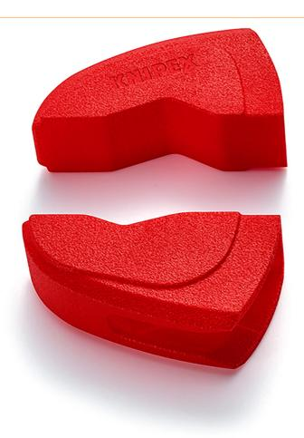
Ideally suited for round workpieces on fittings and other delicate materials thanks to soft gripping surfaces. Entire gripping surface/serration is covered: prevents damage from the aggressive teeth of the gripping jaws. Easy to attach by hand and reliably fixed to the gripper jaws by means of an internal snap-in hook. Smooth gripping surfaces of the jaws (no toothing). Set consisting of 3 pairs of plastic jaws.
