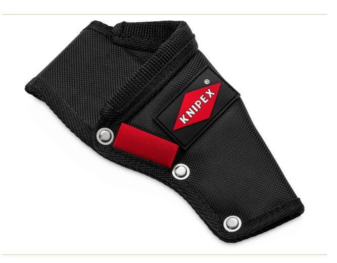
Tool pouch made of durable polyester fabric, with belt loop. Conical cut pouch for 1 to 3 hand tools. Ideally shaped for angled electrician's scissors 95 05 20 SB. Also fits KNIPEX CutiX<sup>®</sup> universal knife or similar slim tools such as electrician's pliers, KNIPEX TwinGrip front gripping pliers, etc. With pin holder. Dimensions (W x H x D): 110 x 40 x 215 mm.
