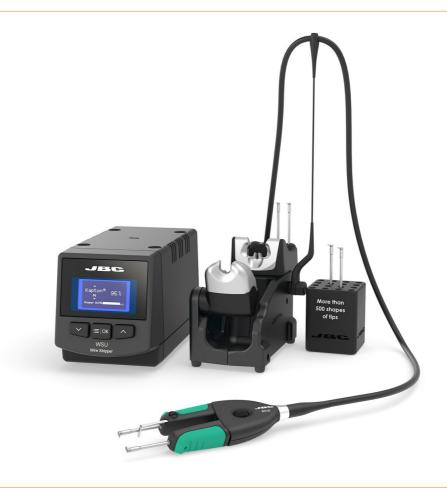
WSS is specially designed for stripping wire insulations made of thermostable materials such as teflon\*, kapton\*, silicone rubber, etc, from 40 to 14 AWG (0.08 to 1.63 mm / 0.0031 to 0.0642 in) with temperatures up to  $800^{\circ}$ C /  $1470^{\circ}$ F.
