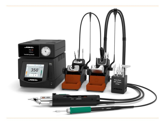
DMU Control Unit manages up to 4 tools simultaneously and is fully compatible with 10 different JBC tools.
