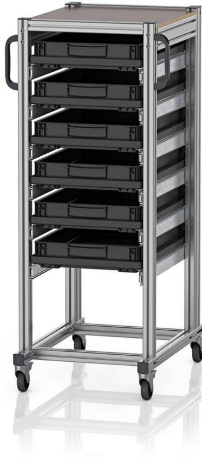
AUER Packaging's ESD system trolley for Euro containers is the ideal solution if the ESD-sensitive contents are frequently required at different work stations. All its parts, including the rollers, are manufactured using electrically conductive plastic and are consequently securely protected from electrostatic charges.
