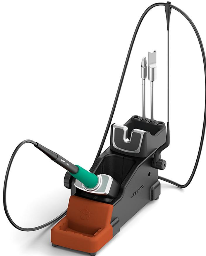
HDS Stand works exclusively with T470 Heavy Duty Handles and HDU Control Unit. Sleep & Hibernation Mode automatically detects the tool in the stand and reduces the tip temperature below the solder melting point. Hibernation cuts off power supply preventing oxidation. As a result, tip life lasts up to 5 times longer.
