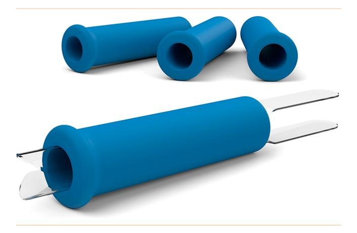
Soft foam grips for T245, T245G and T245P ensure a better manual control of the tool and greater comfort when working.
