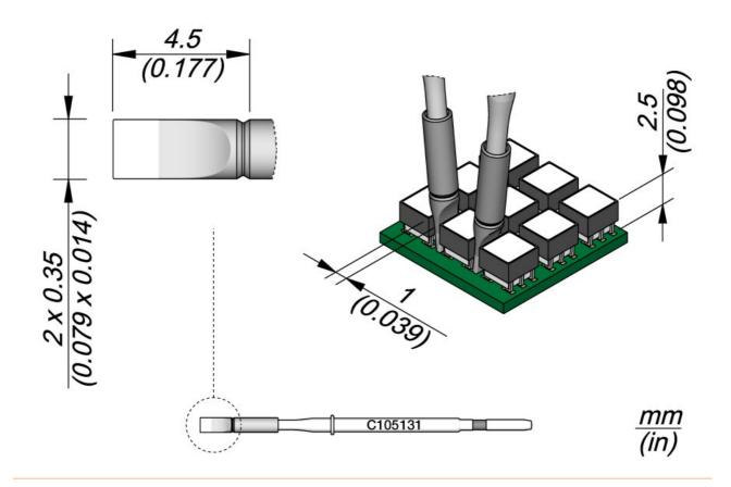
C105 cartridges are the smallest of the JBC range. They are appropriate for soldering and repairing very small-sized components at high precision, even under a microscope. C105 cartridges work with NT105 Nano Soldering Iron and NP105 Nano Tweezers. JBC tips last 5 times longer than other brands thanks to the JBC Most Efficient Soldering System and the Sleep & Hibernation features.
