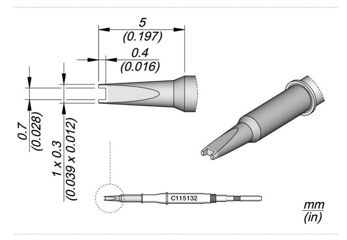
C115132 cartridges are appropriate for desoldering chip components. They work with NT115 Nano Handle and comply with the most demanding regulations. JBC Long Life Tips offer instant heat up, excellent heat transfer and great durability. They last 5 times longer than other brands thanks to the JBC Most Efficient Soldering System and the Sleep & Hibernation features.
