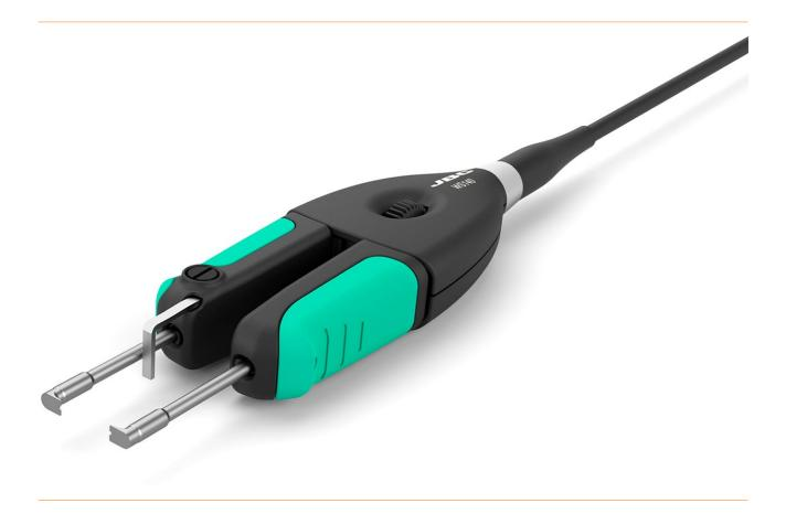
WS140 is specially designed for stripping high temperature cables made of thermostable materials such as Teflon\*, Kapton\*, silicone rubber, etc. from 40 to 14 AWG (0.08 to 1.63 mm / 0.0031 to 0.0642 in) up to 800°C / 1470°F.
