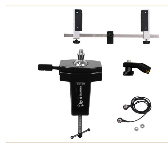
With the SPANNFIX VARIO, PCBs / circuit boards up to a length of 270 mm can be clamped. Due to the infinitely adjustable ball, the PCB can be securely positioned and held in all directions. Quick turning of the PCBs / circuit boards is possible thanks to the adapter, which can be rotated and locked in +/- 45° steps. The adjusting screws with ergonomic handle are smooth-running and facilitate adjustment.
