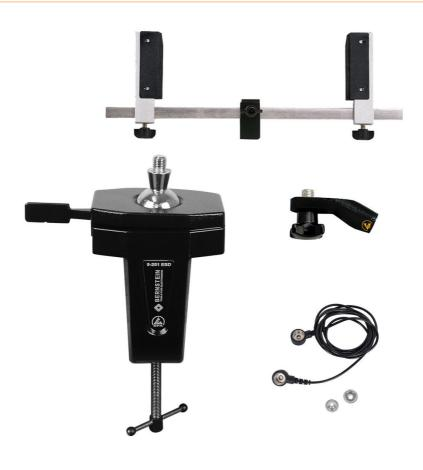
With the SPANNFIX VARIO, PCBs / circuit boards up to a length of 270 mm can be clamped. Due to the infinitely adjustable ball, the PCB can be securely positioned and held in all directions. Quick turning of the PCBs / circuit boards is possible thanks to the adapter, which can be rotated and locked in +/- 45° steps. The adjusting screws with ergonomic handle are smooth-running and facilitate adjustment.
