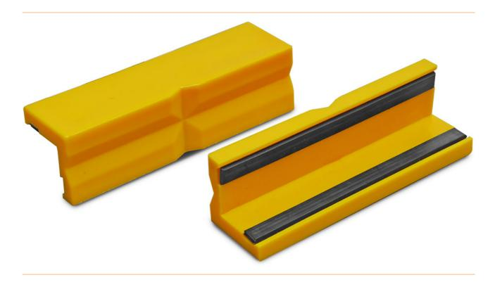
The plastic jaws fit perfectly to any vice with steel jaws due to their double magnetic bar. They protect sensitive components from scratching or damage. Due to the longitudinal and transverse grooves, even round objects can be clamped securely. If the grooves interfere with clamping, the smooth surface of the other side can also be used.
