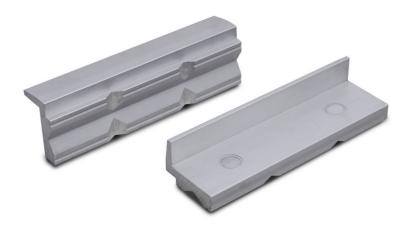
The aluminium jaws sit perfectly on any vice with steel jaws due to their magnets. They protect sensitive components from scratching or damage. Due to the longitudinal and transverse groove, round objects can also be clamped securely.
