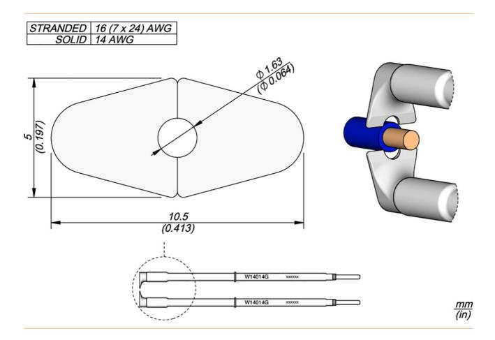
The W14014G is specially designed for stripping high temperature cables made of thermostable materials such as Teflon\*, Kapton\*, silicone rubber etc. with a cross section of 14 AWG (1.63 mm / 0.0642 in).
