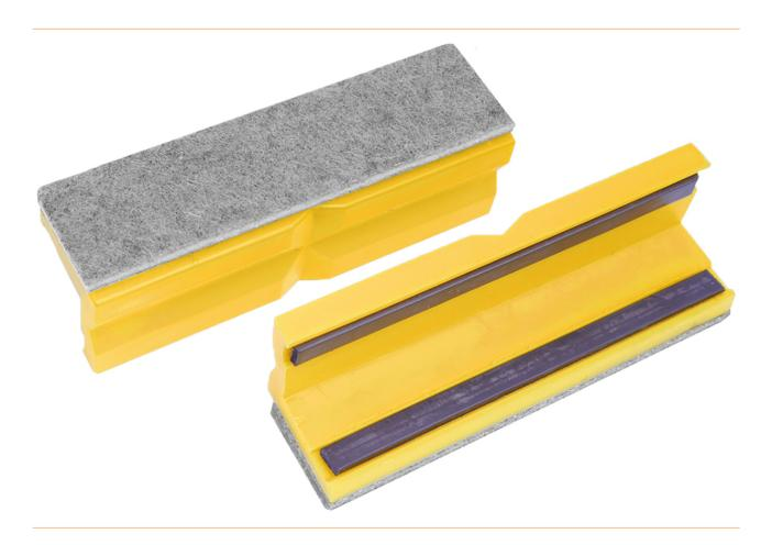
The plastic jaws sit perfectly on any vice with steel jaws due to their double magnetic bar. The lint-free felt layer protects sensitive parts from scratches or damage. Due to the longitudinal and transverse groove, even round objects can be clamped securely.
