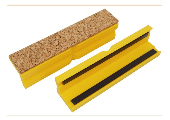
The plastic jaws fit perfectly to any vice with steel jaws due to their double magnetic bar. The elastic and firm cork coating protects sensitive parts from scratches or damage. Due to the longitudinal and transverse groove, even round objects can be clamped securely.
