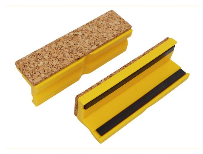
The plastic jaws fit perfectly to any vice with steel jaws due to their double magnetic bar. The elastic and firm cork coating protects sensitive parts from scratches or damage. Due to the longitudinal and transverse groove, even round objects can be clamped securely.
