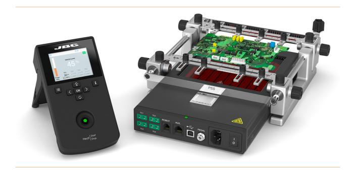
Reduces the risk of thermal shock during rework: The PHSK Small Preheater Set provides the best solution for rework on small / medium PCBAs commonly used in the electronics industry. It has a heating surface of 130 x 135 mm and four TC connections.
