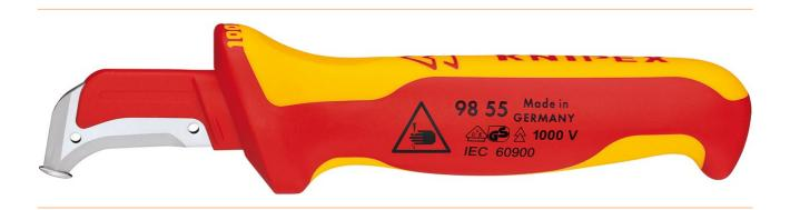
Ergonomically designed handle with pleasant slip guard. More safety due to non-slip soft component. Good power transmission when pulling the knife due to thumb recess and "finger hook" at the end of the handle. Transparent protective cap. stable, fixed hook blade, sickle-shaped. with slide shoe at the tip. no damage to the conductor insulation. Blade: surgical steel, stainless, air-hardened. - Blade length: 38mm - Radius: 23,5mm - VDEtested: Yes
