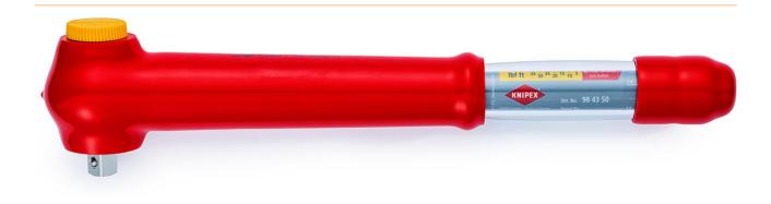
Reversible for tightening left-hand threads. Transparently insulated scale range 5 - 50 Nm. Lockable torque adjustment. Adjustable in 0.25 Nm increments. Very secure fastening of the actuating tools due to screwed locking. Calibration certificate enclosed. - Connecting square: 1/2mm
