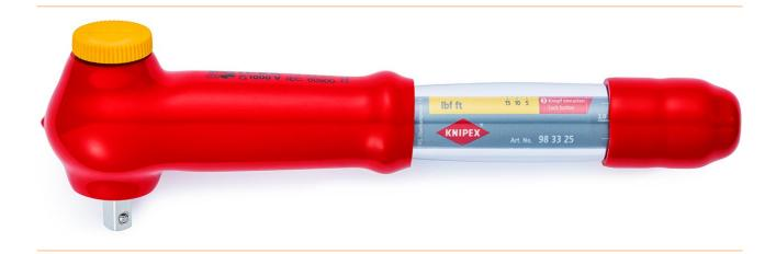
Reversible for tightening left-hand threads. Lockable torque adjustment. Adjustable in 0.25 Nm increments. Very secure fastening of the operating tools due to screwed locking. Calibration certificate enclosed. Transparently insulated scale range 5 - 25 Nm. -
