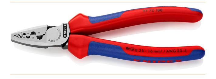
for wire end ferrules: light and slim design. also available as VDE version. easy crimping due to optimised transmission ratio. For crimping wire-end ferrules according to DIN 46228 part 1 + 4 in the range of 0.25 to 16 mm<sup>2</sup>. Crimping in marked half-round profiles for secure connection of sleeve and conductor. Nine particularly deep profiles with conical side surfaces. - Application: Ferrules - Capacity square millimetres: 0.25 - 16.0mm<sup>2</sup> - Number of nests: 9 - AWG: 23 - 5.
