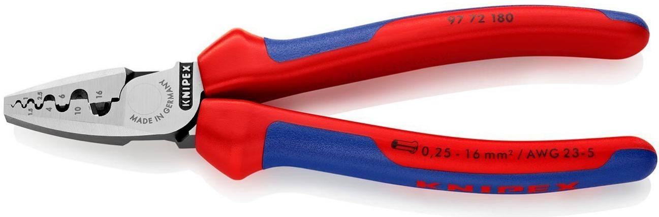
for wire end ferrules: light and slim design. also available as VDE version. easy crimping due to optimised transmission ratio. For crimping wire-end ferrules according to DIN 46228 part 1 + 4 in the range of 0.25 to 16 mm<sup>2</sup>. Crimping in marked half-round profiles for secure connection of sleeve and conductor. Nine particularly deep profiles with conical side surfaces. - Application: Ferrules - Capacity square millimetres: 0.25 - 16.0mm<sup>2</sup> - Number of nests: 9 - AWG: 23 - 5.
