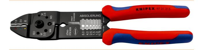
For cutting cables, stripping wires and crimping insulated and uninsulated cable lugs and connectors and open connectors. With threaded holes for cutting copper or brass threaded pins with M 2.6; M 3; M 3.5; M 4 and M 5. Screwed joint for high stability and smooth running. - Application: insulated cable lugs + cable connectors - Capacity square millimetres: 0.5 - 6.0mm<sup>2</sup> - Number of nests: 3 - AWG: 20 - 10
