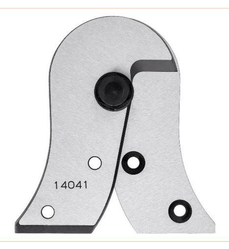
Replacement cutter head for 95 71 600 / 95 77 600 For wire ropes and round bars, Cu and Al cables. Suitable for cutting overhead cables with strain relief wire. Angled cutting tips enable cutting of individual rope strands. Optimum transmission ratio for high cutting performance. Bolted cutter head, replaceable. Low weight.
