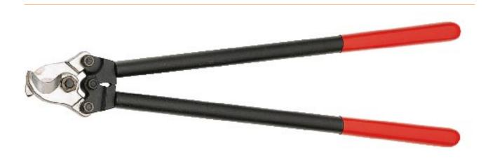
For cutting copper and aluminium cables, solid and stranded. Not suitable for steel wire and wire ropes. Hardened cutting edges with precision grinding. Cuts smoothly and cleanly without crushing. Favourable transmission ratios due to toggle lever mechanism. Pinch protection prevents crushing injuries. Adjustable screw joint. Bolted cutter head, replaceable. - Cutting value Cu-cable, stranded: 150mm² - Cutting value Cu-cable, stranded: Ø 27mm - AWG: 5 / 0
