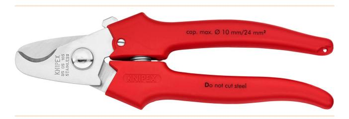
Not suitable for steel wire and hard-drawn copper conductors. Hardened cutting edges with precision grinding. No crushing, low deformation of the cable. Pinch protection prevents crushing injuries. Adjustable screw joint. For cutting cables Ø 10 mm / 24 mm<sup>2</sup>. With opening spring and ratchet. Cutting edges made of stainless steel. oil-hardened and tempered. - Cutting value Cu-cable, stranded: 24mm<sup>2</sup> - Cutting value Cu-cable, stranded: Ø 10mm - AWG: 3
