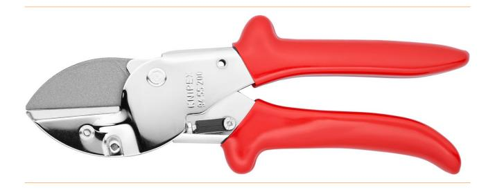
Pulling cut against a firm base for crush-free cutting of soft materials such as rubber profiles, PVC, leather, wood, hoses, etc.. Cuts flat material up to max. 40 mm width and 7.5 mm height. Cutting capacity for round material up to ø 25 mm. Robust, replaceable blade. With opening spring and ratchet.
