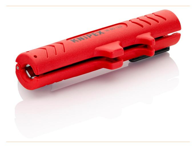
Suitable for stripping and stripping all common round and wet room cables from  $\emptyset$  8.0 to 13.0 mm (e.g. NYM cable 3 x 1.5 mm<sup>2</sup> to 5 x 2.5 mm<sup>2</sup>). Also for use in junction or distribution boxes. Double-shell, hinged stripping tool. With opening spring and ratchet. Fastening clip for safe storage. - Stripping values (diameter):  $\emptyset$  8 - 13mm - Cable type: round cable, e.g.: 3 x 1.5 mm<sup>2</sup> to 5 x 2.5 mm<sup>2</sup>.
