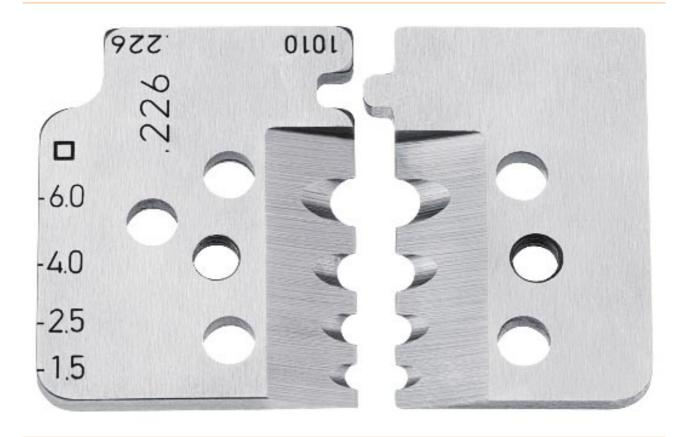
1 set of replacement blades for 12 12 11 Positive stripping even of hard-to-remove insulating materials made of PTFE, silicone, Radox®, Kapton® and rubber; also multi-layered. A second pair of blades reliably holds the remaining insulation. Interchangeable shaped blades precisely matched to the respective conductor cross-section. With adjustable length stop for equal stripping lengths when working in series.
