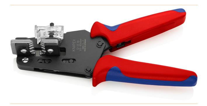
Form-fitting stripping even of hard-to-remove insulating materials made of PTFE, silicone, Radox®, Kapton® and rubber; also multi-layered. A second pair of blades reliably holds the remaining insulation. Interchangeable shaped blades precisely matched to the respective conductor cross-section. With adjustable length stop for equal stripping lengths when working in series. - Stripping values square millimetres:  $2.5 / 4.0 / 6.0 / 10.0 \text{mm}^2$  - AWG: 13 - 7
