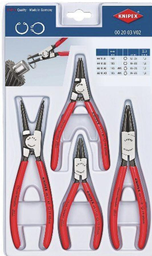
Sturdy plastic packaging; also suitable for further storage of the pliers. Equipped with common circlip pliers for inner and outer rings. 4-piece set. Scope of delivery: 1 x 44 11 J1 KNIPEX circlip pliers for inner rings in bores ( $\varnothing$  12 - 25 mm), 1 x 44 11 J2 KNIPEX circlip pliers for inner rings in bores ( $\varnothing$  19 - 60 mm), 1 x 46 11 A1 KNIPEX circlip pliers for outer rings on shafts, 1 x 46 11 A2 KNIPEX circlip pliers for outer rings on shafts,
