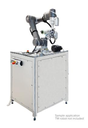
The TM Mobile Workstation with integrated work area - can be used both individually and flexibly. The control system is stowed inside the workstation and is easily accessible through side openings. Optionally with built-in PLC, compressed air connections and TP-100-1 TM Kit.
