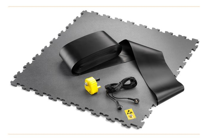
The 7 mm ESD X-Log grounding tile is used every 50 square metres. The grounding tile can be connected to the ground via a grounding cable on a grounding plug or grounding rail, according to the installation instructions.
